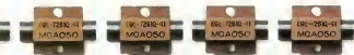
feel with sensors and accelerometers. We place these devices throughout the body—in all strategic points of the dummy—to monitor the force of impact these areas receive in a crash.
